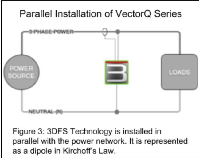
The full installation requires the temporary removal of the front panel. Three Flex-coil current transformers (1 for each phase) are installed around the incoming phases. A three block fuse (1 for each phase) is installed into the panel for a voltage connection. If neutral and/or ground wires are available, they are also wired to the power controller. The panel can then be returned and the installation is complete.
