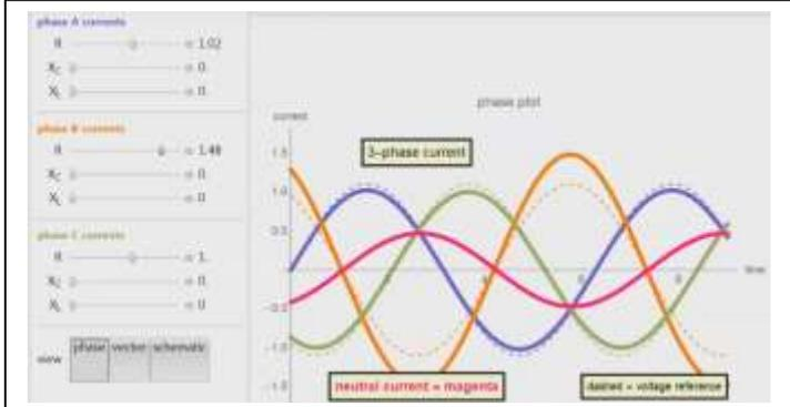
When any phase shift (Current leading or lagging the Voltage) is present, a proportional increase in Neutral Current will result.
