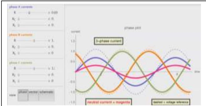
When a decreased current imbalance is introduced on one phase, the Neutral Current is increased in proportion.
