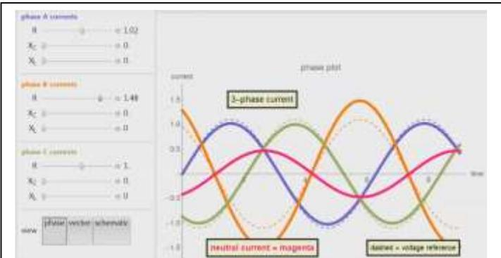
When an increased current imbalance is introduced on one phase, the Neutral Current is still increased in proportion.
