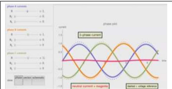
When the Current and Voltage is synchronized and balanced across all phases Neutral Current does not exist.
