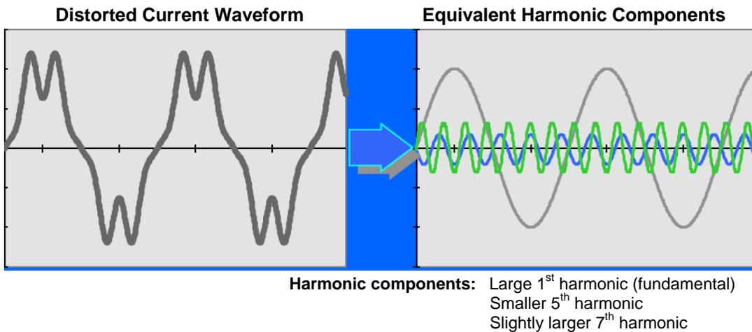
**Figure 2. Distorted waveform composed of fundamental and 3<sup>rd</sup> harmonic**
