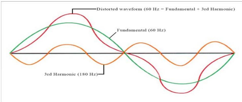
**Figure 1. Harmonic distortion of the electrical current waveform**
